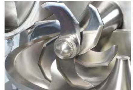
Cutting head with 6 standard knives BE-GW Steffens (Germany).
