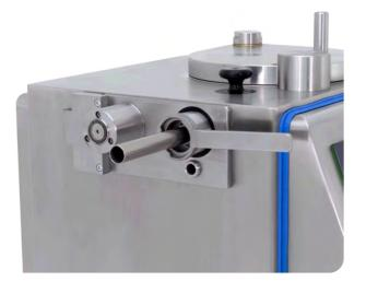
**FP30e: filling/stuffing and portioning** Single or continuous operation, programmable number of portions with automatic stop.
