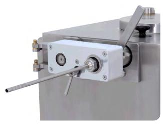
**FP30t: automatic digital twister/linker** Rotates the nozzle/horn between each portion. Number of turns adjustable from 1 to 15 turns.
