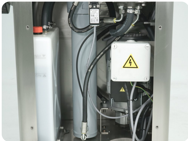
Powerful hydraulic system. Transparent oil reservoir, completely independent.
